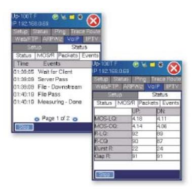
The VoIP Call Expert emulates an IP phone and can place and receive calls using SIP or H.323 protocols. Comprehensive Codec support and call destination options verify voice encoding and translation provisioning. Real time evaluation of subjective voice quality (MOS and R-factor) is made possible using the patented Telchemy test method which has been integrated into all VePAL test sets.
